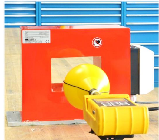
Illustration 4: Whole body exposure measurement of an air coil
