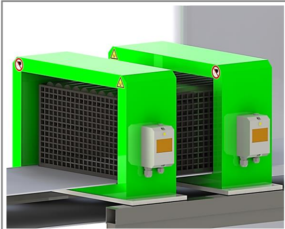
Image: Coil module in Helmholtz configuration, horizontal orientation of the components, suitable for elongated parts lying in the washing basket.
