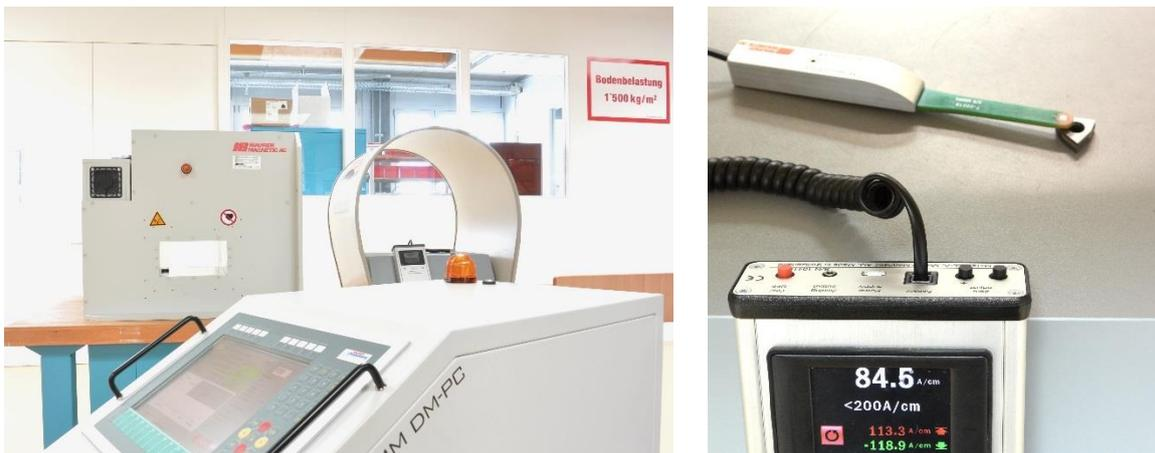
Figure 4: Maurer Magnetic VE-2 Coil Module with 260kA/m, DM-P Power Module and measuring device M-Test LL
